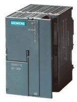
SIPLUS S7-300 IM 365 based on 6ES7365-0BA01-0AA0 with conformal coating, -25...+60  $^{\circ}$ C, connection IM 365 for connection of an extension rack, without communications bus, 2 modules+ connecting cable 1 m
