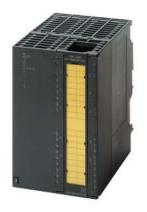
\*\*\*spare part\*\*\* SIPLUS S7-300 SM 326F DQ8 based on 6ES7326-2BF41-0AB0 with conformal coating, -25...+60 °C, digital output F-DQ 8x 24 V DC/2A PM fail-safe digital output sinking-sourcing up to category 4 (EN 954-1), SIL 3 (IEC 61508)
