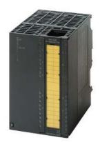
SIPLUS S7-300 SM 326F DQ8 based on 6ES7326-2BF41-0AB0 with conformal coating, -25...+60 °C, digital output F-DQ 8x 24 V DC/2A PM fail-safe digital output sinking-sourcing up to category 4 (EN 954-1), SIL 3 (IEC 61508)
