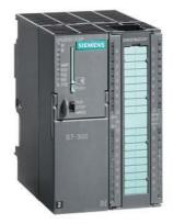
SIPLUS S7-300 CPU 313C-2DP based on 6ES7313-6CG04-0AB0 with conformal coating, -25...+70  $^{\circ}$ C, compact CPU with MPI, 16 DI/16 DQ, 3 high-speed counters (30 kHz), integrated DP interface, integrated power supply 24 V DC, work memory 128 KB, front connector (1x 40-pole) and Micro Memory Card required
