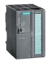
SIPLUS S7-300 CPU 312C based on 6ES7312-5BF04-0AB0 with conformal coating, -25...+70 °C, compact CPU with MPI, 10 DI/6 DQ, 2 high-speed counters (10 kHz) integrated power supply 24 V DC, work memory 64 KB, front connector (1x 40-pole) and Micro Memory Card required
