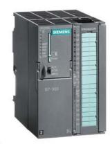
\*\*\*spare part\*\*\* SIPLUS S7-300 CPU 312C based on 6ES7312-5BF04-0AB0 with conformal coating, -25...+60 °C, compact CPU with MPI, 10 DI/6 DQ, 2 high-speed counters (10 kHz) integrated power supply 24 V DC, work memory 64 KB, front connector (1x 40-pole) and Micro Memory Card required
