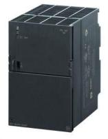
SIPLUS S7-300 PS 307 10 A based on 6ES7307-1KA02-0AA0 with conformal coating, -25...+70  $^{\circ}\text{C}$ , stabilized power supply PS 307 input: 120/230 V AC output: 24 V DC/10 A
