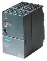
SIPLUS S7-300 PS 305 based on 6ES7305-1BA80-0AA0 with conformal coating, -25...+70 °C, stabilized power supply input: 24-110 V DC output: 24 V DC/2 A
