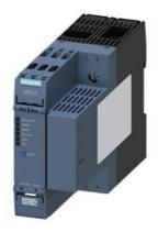
DC load monitoring relay for PROFINET, max. 1x63 A DC, max. 800 V Width: 45.0 mm Monitoring for violation of upper and lower limit of current, voltage and power; Energy consumption counter, energy recovery counter, switching cycle counter, operating hours counter, warning and alarm thresholds, automatic or manual reset, ON delay 0-999.0 sec, OFF delay 0-999.0 sec, automatic reclosing delay 0-999.0 sec Supply voltage: 24 V DC 1 changeover contact, screw terminal
