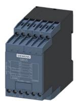
voltage reducer module for insulation monitoring relay 3UG4583 for expanding the supply voltage range to 690 V AC and 1000 V DC screw terminal
