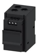
Current/voltage measuring module for dry-running protection of centrifugal pumps in hazardous areas; set current 10 ... 115 A, voltage measurement up to 690 V, width 55 mm, straight-through transformer
