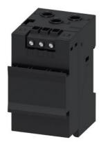
Current/voltage measuring module for dry-running protection of centrifugal pumps in hazardous areas; set current 3 ... 40 A, voltage measurement up to 690 V, width 45 mm, straight-through transformer
