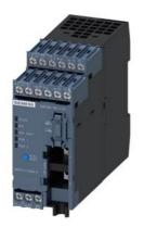
Basic unit SIMOCODE pro V EIP, EtherNet/IP, medium redundancy DLR, Web server, transmission rate 100 Mbps, 2 x bus connection via RJ45, 4I/3O freely parameterizable, Us: 110...240 V AC/DC, input for thermistor connection Monostable relay outputs, expandable by extension modules
