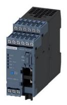
Basic unit SIMOCODE pro V EIP, EtherNet/IP, medium redundancy DLR, Web server, transmission rate 100 Mbps, 2 x bus connection via RJ45, 4l/30 freely parameterizable, Us: 24 V DC, input for thermistor connection Monostable relay outputs, expandable by extension modules
