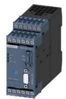
Basic unit SIMOCODE pro V MR, MODBUS RTU interface 57.6 Kbps, RS 485, 4I/30 freely parameterizable, Us: 24 V DC, input for thermistor connection Monostable relay outputs, expandable by extension modules
