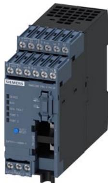
Basic unit SIMOCODE pro V PN GP , Ethernet/PROFINET IO, PN system redundancy, OPC UA server, Web server, transmission rate 100 Mbps, 2 x bus connection via RJ45, 4 I/3 Q freely parameterizable, Us: 24 V DC, input for thermistor connection Monostable relay outputs, expandable by 1 extension module(DM, TM, EM)
