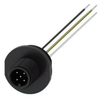
Accessory for position switches 3SE51/52; M12 connector 5-pole, for M20 x 1.5; Pin1=Brown cable, Pin2=White cable, Pin3=Yellow-green cable, Pin4=Black cable, Pin5=Gray cable. Suitable for wiring sensors that are to be connected to all SIMATIC ET200 compact block I/O modules .
