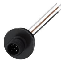
accessories for position switch device plug (5-pole), M12, for M20 x 1.5 for 125 V, 4 A on Pin 5 a gray line no yellow/green line for PE as for 3SY3128  $\,$
