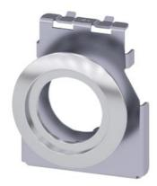
Adapter for installation of actuators and signaling units, 22 mm, in a mounting drill hole 30.5 mm, Metal, shiny, with seal
