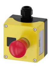
AS-Interface enclosure for command devices 22 mm, round, enclosure material metal, enclosure top part yellow, 1 control point metal, recess for label, A=EMERGENCY STOP mushroom pushbutton red, 40 mm, rotate-to-unlatch, 1 NC, 1 NC, spring-type terminal, floor mounting, AS-i shaped cable Direct entry top/right, label enclosed
