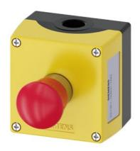
Enclosure for command devices, 22 mm, round, Enclosure material metal, Enclosure top part yellow, 1 control point metal, A=EMERGENCY STOP mushroom pushbutton red, 40 mm, rotate-to-unlatch, Control point in center, 2 NC, screw terminal, floor mounting, 1xM20 each on top and bottom
