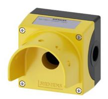
Enclosure for command devices, 22 mm, round, metal enclosure, yellow enclosure top, with protective collar, rotated by  $90^\circ$ , for 5 padlocks, for horizontal installation, and mushroom diameter 60 mm, 1 control point, without equipment, floor mounting, left and right each 1xM20
