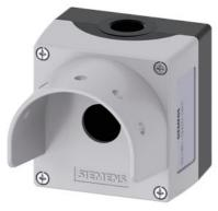
Enclosure for command devices, 22 mm, round, Enclosure material metal, enclosure top part gray, with protective collar for 5 padlocks, and mushroom diameter 60 mm, 1 control point, without equipment, floor mounting, 1xM20 each on top and bottom
