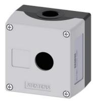
Enclosure for command devices, 22 mm, round, Enclosure material metal, enclosure top part gray, 1 control point, without equipment, Recess for labels, floor mounting, 1xM20 each on top and bottom
