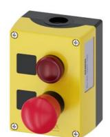
Enclosure for command devices, 22 mm, round, Enclosure material plastic, Enclosure top part yellow, 2 control points plastic, B=Indicator light red, LED 24 V, screw terminal, label without inscription, A=Emergency stop 40 mm rotate-to-unlatch, label without inscription, 1 NO, 1 NC, 1 NC, screw terminal, floor mounting, 1xM20 each on top and bottom, Labels enclosed
