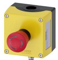
Enclosure for command devices, 22 mm, round, enclosure material plastic, enclosure top part yellow, 1 control point plastic, A=EMERGENCY STOP mushroom pushbutton red, 40 mm, rotate-to-unlatch, illuminated, 2x 1 NC, LED white 24 V, spring-type terminal, floor mounting, M12 connector (8-pole) bottom, insulated reserve conductors Pin assignment: PIN1=11, PIN2=12, PIN3=21, PIN4=22, Pin5=n.c., Pin6=n.c., Pin7=ground LED, PIN8=LED, one connection at 1 input F-DI, one connection at 1 output F-DQ
