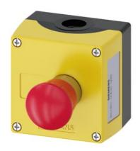
Enclosure for command devices, 22 mm, round, enclosure material plastic, enclosure top part yellow, 1 control point, A=EMERGENCY STOP mushroom pushbutton red, metal, 40 mm, rotate-to-unlatch, 1 NO, 1 NC, 1 NC, spring-type terminal, floor mounting, support terminal, without label, 1xM20 each on top and bottom
