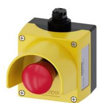
AS-Interface enclosure for command devices 22 mm, round, Enclosure material plastic, Enclosure top part yellow, with protective collar, 1 control point plastic, A=EMERGENCY STOP mushroom pushbutton red, 40 mm, rotate-to-unlatch, 1 NC, 1 NC, spring-type terminal, floor mounting, Insulation displacement system on top
