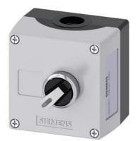
Enclosure for command devices, 22 mm, round, enclosure material plastic, enclosure top part gray, 1 control point, A = selector switch, black, metal 2 switch positions, momentary contact, 1 NO, spring-type terminal, floor mounting, support terminal, without label, 1xM20 each on top and bottom
