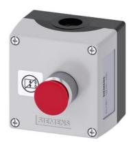
Enclosure for command devices 22 mm, round, enclosure material plastic, enclosure top part gray, 1 control point, A = Push-pull switch, red, metal, 30 mm, 1 NC, spring-type terminal, floor mounting, support terminal, customized label, top and bottom 1xM20 each, Label glued in
