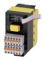
SIRIUS ACT with PROFINET: fail-safe interface module with 4 DI, 1 DQ (24 V DC), 1 AI (12-bit A/D resolution), 24 V DC, spring-loaded terminal, front plate mounting, 1 to 20 terminal modules connectable
