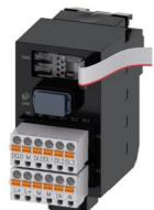
SIRIUS ACT with PROFINET: standard interface module with extended inputs and outputs 24 V DC, spring-loaded terminal, front plate mounting, 1 to 20 terminal modules connectable, with additional 1 DQ + 4 DI + 1 AI
