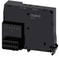
Electronics module for IO-Link, black, 8 inputs/outputs, user-programmable, default 6 DI/2 DQ, Spring-type terminal (Push-in), for front plate mounting
