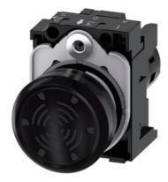
acoustic signal device, compact, 22 mm, round, plastic, black, continuous tone 4.5 kHz, lP69, sound pressure 75+/-10% dB/10 cm, with holder, operating voltage 230 V AC, screw terminal
