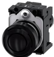
acoustic signal device, compact, 22 mm, round, plastic, black, Continuous tone 2.4 kHz, IP40, Sound pressure min. 80 dB/10 cm, with holder, Operating voltage 230 V AC, screw terminal
