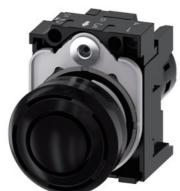
acoustic signal device, compact, 22 mm, round, plastic, black, Continuous tone 2.4 kHz, IP40, Sound pressure min. 80 dB/10 cm, with holder, Operating voltage 24 V AC/DC, screw terminal
