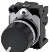
Potentiometer, compact, 22 mm, round, plastic, black, 4.7k ohm, with holder, screw terminal
