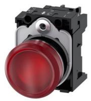
Indicator lights, 22 mm, round, metal, shiny, red, lens, smooth, with holder, LED module with integrated LED 230 V AC, screw terminal
