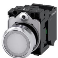
Illuminated pushbutton, 22 mm, round, metal, shiny, white, pushbutton, flat, momentary contact type, with holder, 1 NO, LED module with integrated LED 110 V AC, Spring-type terminal
