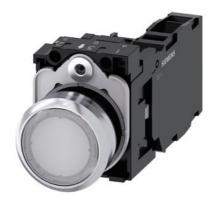
Illuminated pushbutton, 22 mm, round, metal, shiny, white, pushbutton, flat, momentary contact type, with holder, 1 NO+1 NC, LED module with integrated LED 110 V AC, screw terminal
