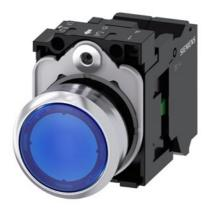
Illuminated pushbutton, 22 mm, round, metal, shiny, blue, pushbutton, flat, momentary contact type, with holder, 1 NO, LED module with integrated LED 110 V AC, Spring-type terminal
