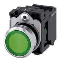
Illuminated pushbutton, 22 mm, round, metal, shiny, green, pushbutton, flat, momentary contact type, with holder, 1 NO, LED module with integrated LED 110 V AC, Spring-type terminal
