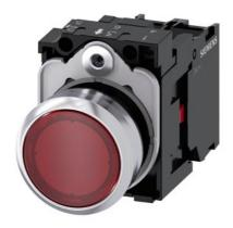
Illuminated pushbutton, 22 mm, round, metal, shiny, red, pushbutton, flat, momentary contact type, with holder, 1 NC, LED module with integrated LED 110 V AC, screw terminal
