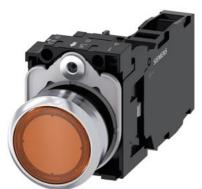
Illuminated pushbutton, 22 mm, round, metal, shiny, amber, pushbutton, flat, momentary contact type, with holder, 1 NO+1 NC, LED module with integrated LED 110 V AC, screw terminal
