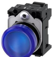
Indicator lights, 22 mm, round, metal, shiny, blue, lens, smooth, with holder, LED module with integrated LED 24 V AC/DC, Spring-type terminal
