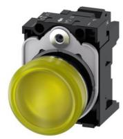
Indicator lights, 22 mm, round, metal, shiny, yellow, lens, smooth, with holder, LED module with integrated LED 24 V AC/DC, Spring-type terminal
