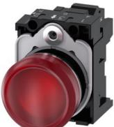
Indicator lights, 22 mm, round, metal, shiny, red, lens, smooth, with holder, LED module with integrated LED 24 V AC/DC, Spring-type terminal
