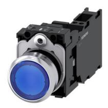
Illuminated pushbutton, 22 mm, round, metal, shiny, blue, pushbutton, flat, momentary contact type, with holder, 1 NO+1 NC, LED module with integrated LED 24 V AC/DC, Spring-type terminal
