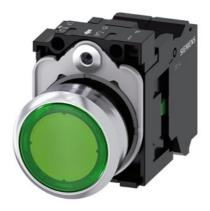
Illuminated pushbutton, 22 mm, round, metal, shiny, green, pushbutton, flat, momentary contact type, with holder, 1 NO, LED module with integrated LED 24 V AC/DC, Spring-type terminal
