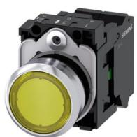
Illuminated pushbutton, 22 mm, round, metal, shiny, yellow, pushbutton, flat, momentary contact type, with holder, 1 NO, LED module with integrated LED 24 V AC/DC, Spring-type terminal
